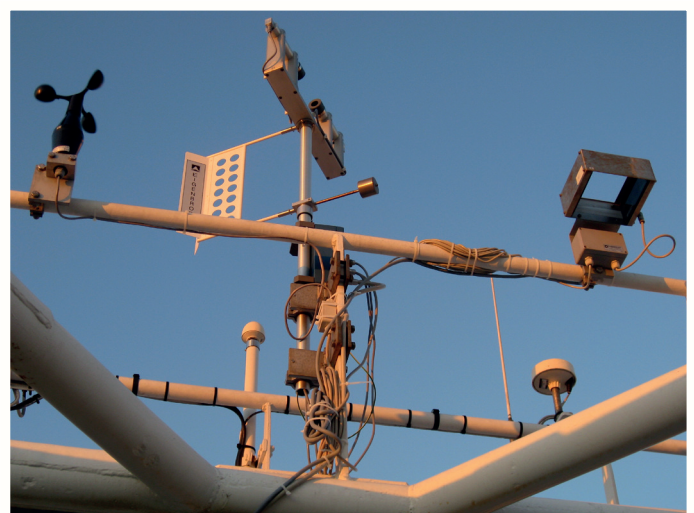
Fig. 1: The automatic measurement system ODM470-400 consisting of the ODM470 (middle), the cup anemometer (left) and the precipitation detector IRSS88 (right) in the highest parts of the ships mast onboard R/V "Polarstern". The ODM470 rotates 360° into the local wind direction by aid of a wind vane.
