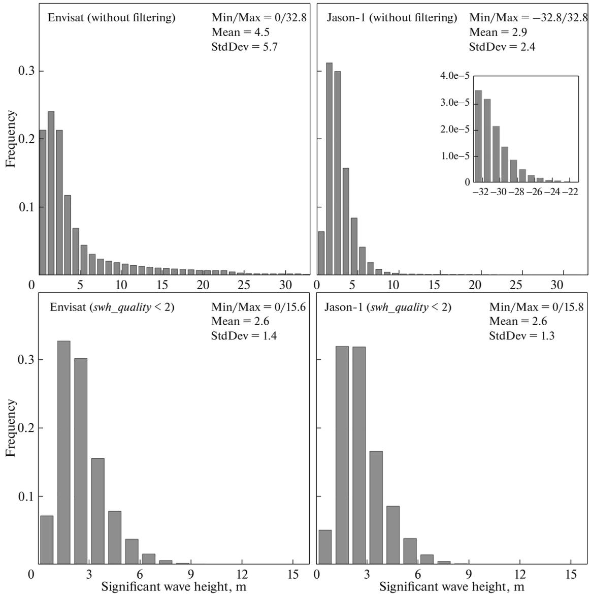
Fig. 2. Histograms of significant wave heights according to data of Envisat (left) and Jason-1 (right) without filtering (upper panel) and with minimal filtering  $swh\_quality < 2$  (lower panel). Main statistical characteristics for 2003 are given in the upper right corner.
