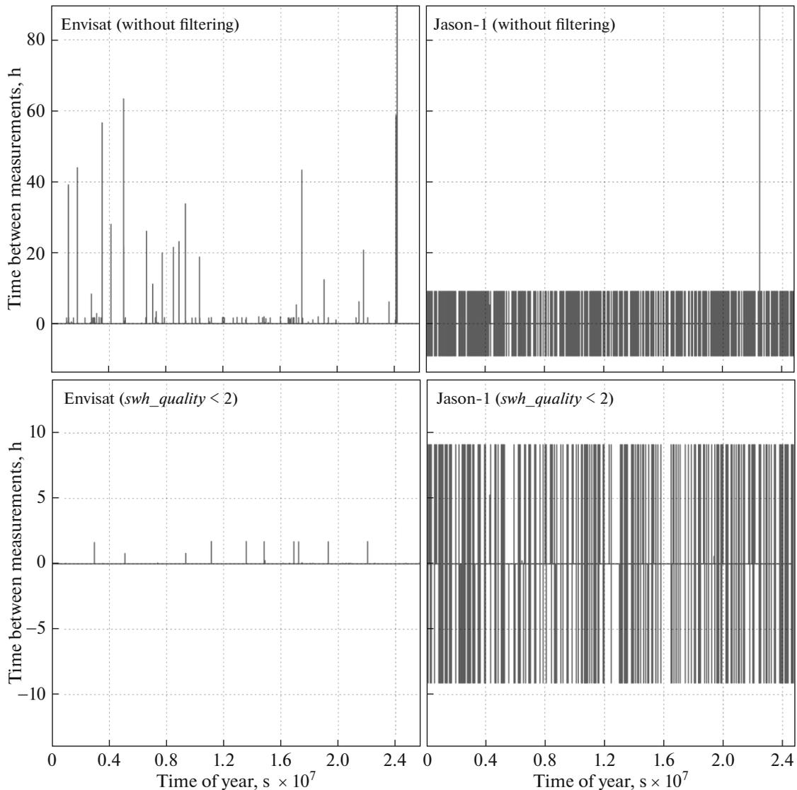
**Fig. 1.** Time difference between consecutive measurements (parameter *dtime*) in data of Envisat (left) and Jason-1 (right) without filtering (upper panel) and with minimal filtering *swh\_quality* < 2 (lower panel), 2003.
