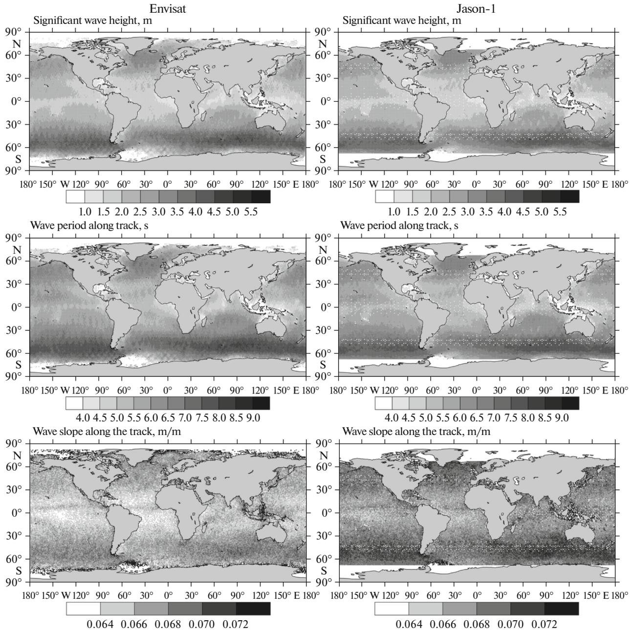
**Fig. 3.** Average annual significant wave heights, periods, and wave slopes for Envisat (left panel) and Jason-1 (right panel) missions after filtering by  $swh\_quality < 2$  and  $5 \text{ km} < distance < 8 \text{ km}$ . This example is based on 2003 data.
